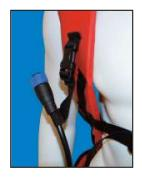
When disconnected from Screed, always attach the cable to your harness to prevent it from falling into concrete or getting tangled onto surrounding element.
